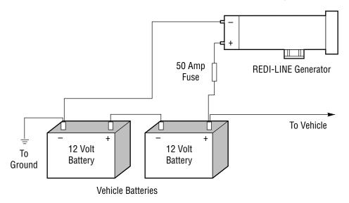
If the load requirement is not heavy (intermittent hand tool use or light loads for a long period of time) the vehicle battery and charging system should handle both the vehicle and additional generator demand.
