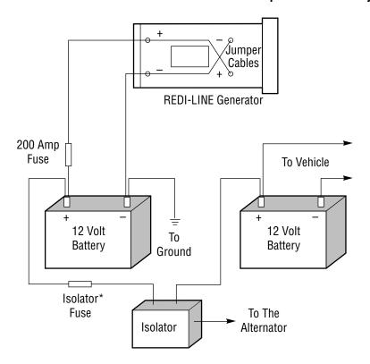
If the load requirement is not heavy (intermittent hand tool use or light loads for a long period of time) install one or more auxiliary deep cycle batteries. The auxiliary battery should be isolated from the vehicle battery using a battery isolator. The battery isolator is a one way path so both batteries are charged by the vehicle but one battery cannot discharge the other. This will ensure the vehicle battery is always charged and you will be able to start your vehicle.
