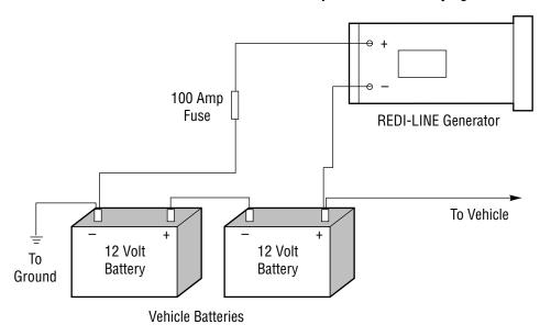
If the load requirement is not heavy (intermittent hand tool use or light loads for a long period of time) the vehicle battery and charging system should handle both the vehicle and additional generator demand.
